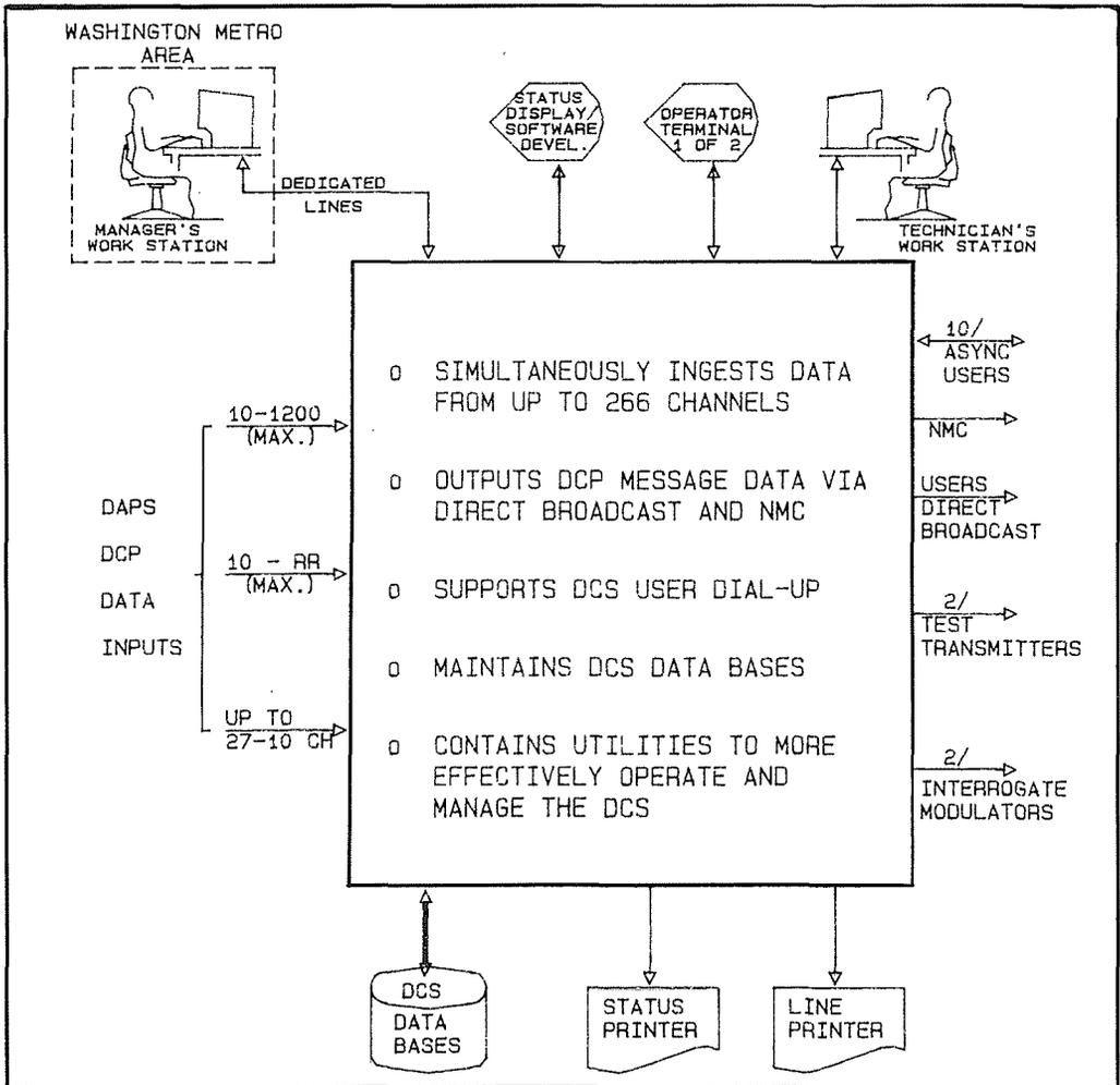
FIG.5 New GOES DCS ground system capabilities
