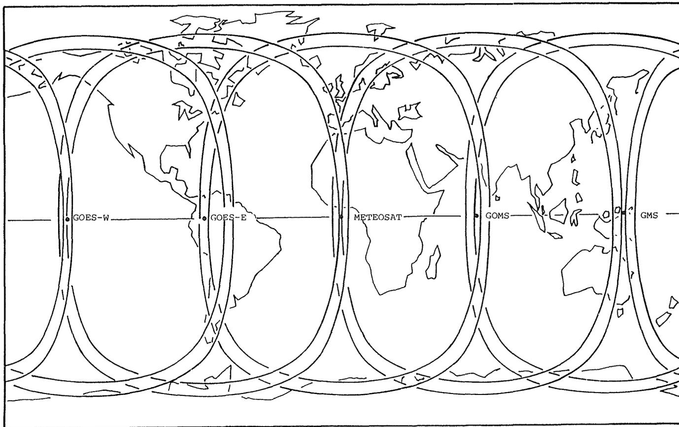
FIG.2 Geostationary meteorological satellite radio footprints
