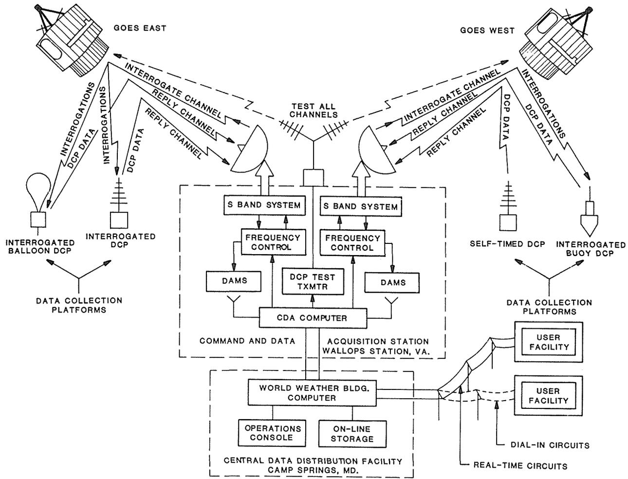
FIG.3 GOES DCS schematic
