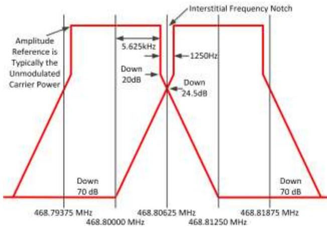
FIGURE 1. FCC 12.5 kHz Emission Mask D.
