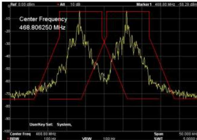
FIGURE 2. 2 NBFM signals with FCC emission masks.
