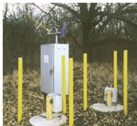
Figure 23: Example of USGS Ground Water Well with GOES DCP
