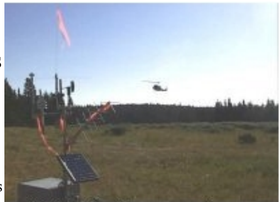
Figure 25: RAWS Unit with GOES DCP on the Bull Elk Park Fire
