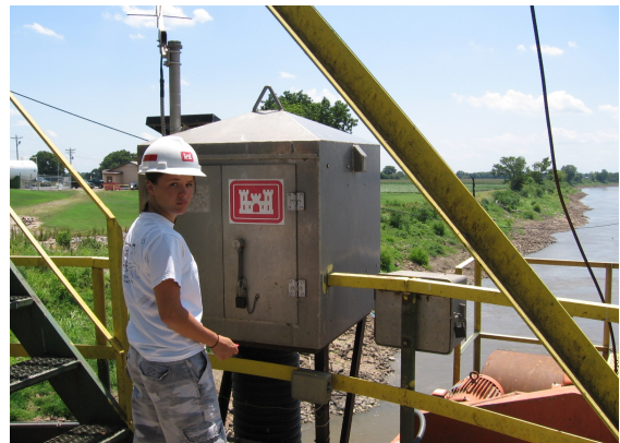
Figure 26: Example of Corps of Engineer's Gage with GOES DCP
