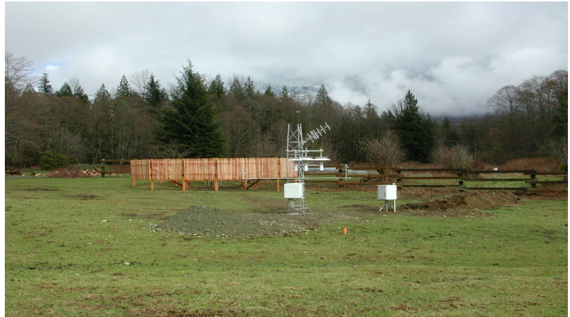
Figure 20: U.S. Climate Reference Site with GOES DCP in the North Cascades National Park, State of Washington
