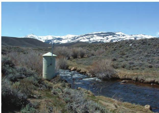
22: Example of USGS Streamgage with GOES DCP
