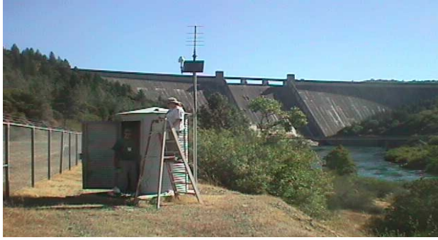
Figure 2. DCP Located Below Reservoir
