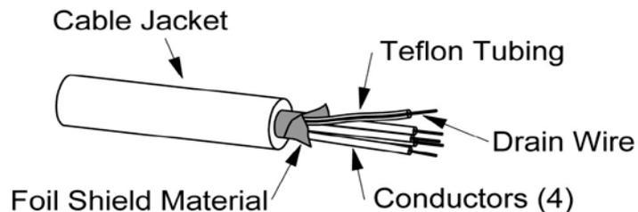
Teflon Tubing (AKA "spaghetti tubing") is often used on the end of a Drain Wire to prevent shorting out other lines, etc...
