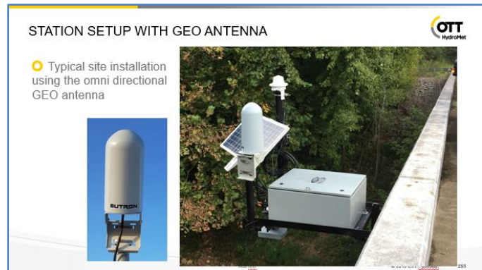
Figure 39: OTT/Sutron SatLink Installation with a GEO Antenna
