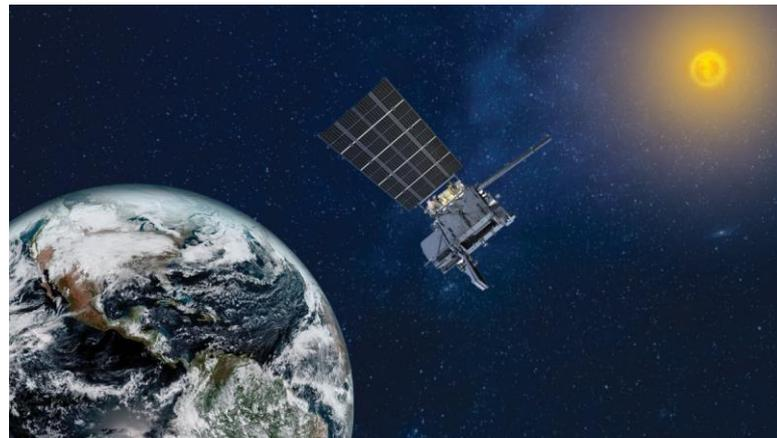
**The Geo Program is evaluating the potential to increase the operational life of the GOES-R series spacecraft by ceasing North-South Station-keeping (NSSK) as spacecraft approach end of life**
