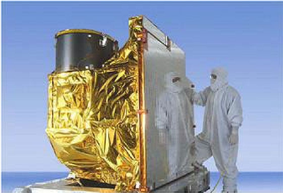
Figure 1: A view of the Advanced Baseline Imager (ABI), from [1].
