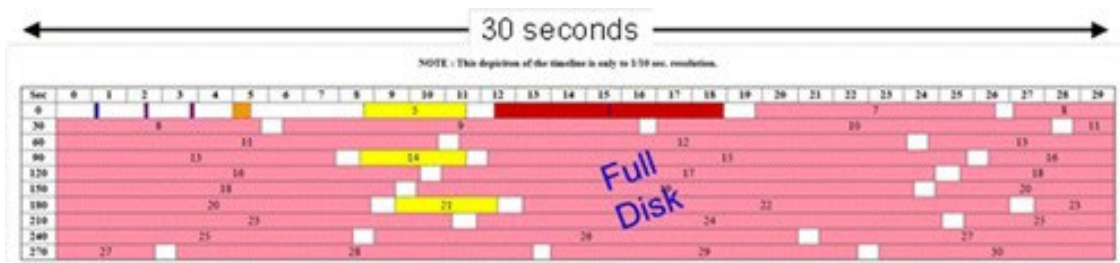
Figure 5: ABI Continuous Full Disk (scan mode 4) timeline diagram. This timeline covers 5 min. Colors same as Figure 4. There are no PACUS or mesoscale scenes in this timeline.
